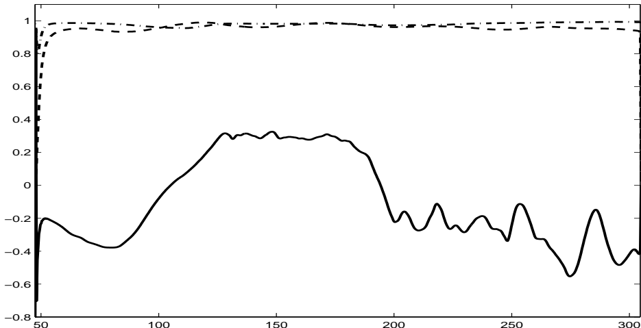
Figure 4.5: Correlation coefficient between -G_1/2 and \mu_{12}/\bar{\rho} \partial_1(\bar{\rho}k) (—), between -G_2/2 and \mu_{12}/\bar{\rho} \partial_2(\bar{\rho}k) (---), and between -G_1/2 and +G_2/2 (-·-) as a function of the streamwise coordinate.
